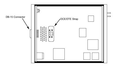
Figure 9. Setting the DCE/DTE Strap
